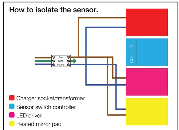
Rewire the mirror as shown in the diagram above. HIB recommends that all electrical bathroom products should only be fitted by a suitably qualified, Part P registered electrician.
